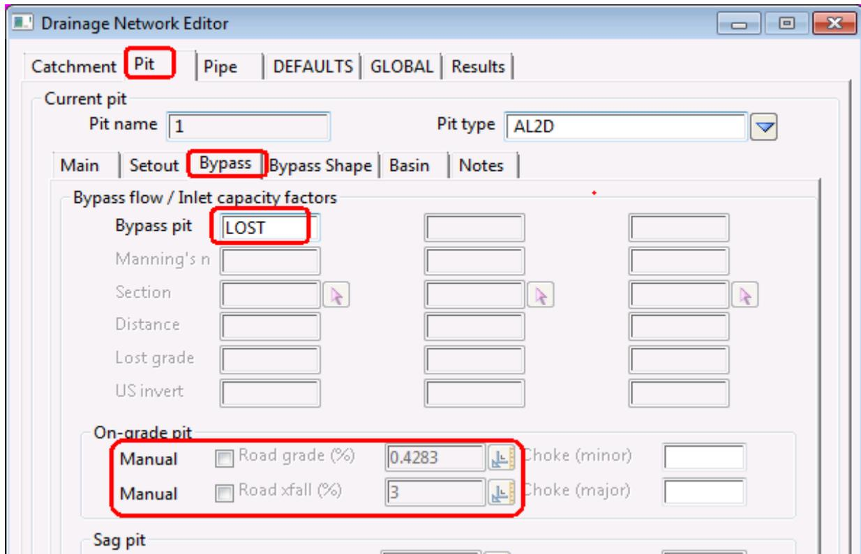
The downstream pit will now show in the **Bypass pit** field. If the bypass string does not go to another inlet (the network outlet is never an inlet) then the **Bypass pit** will be marked as **LOST**.
