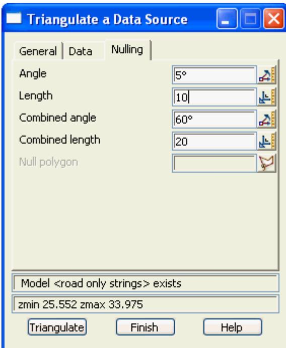
**Length** - Select a length just greater than the width of half the road so that the tin will not be nulled from the end of the roads.
