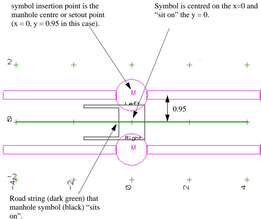
To create the symbol in 12d draw the left pit symbol in a model by itself. The pit should “sit on” the zero “y” grid line. A 900 wide by 600 long inlet with a 1.2m lintel is shown above.
