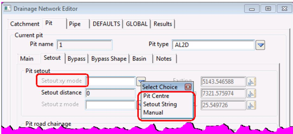
The following example of a channel ip point is given below. The setout modes are set, the cover and grate level modes are set and the ku (losses) are set. Finally, the inlet capacity is set to an on-grade pit with 200% inlet capacity so that even in a major storm with a choke factor of 0.5 it will still have 100% inlet capacity.
