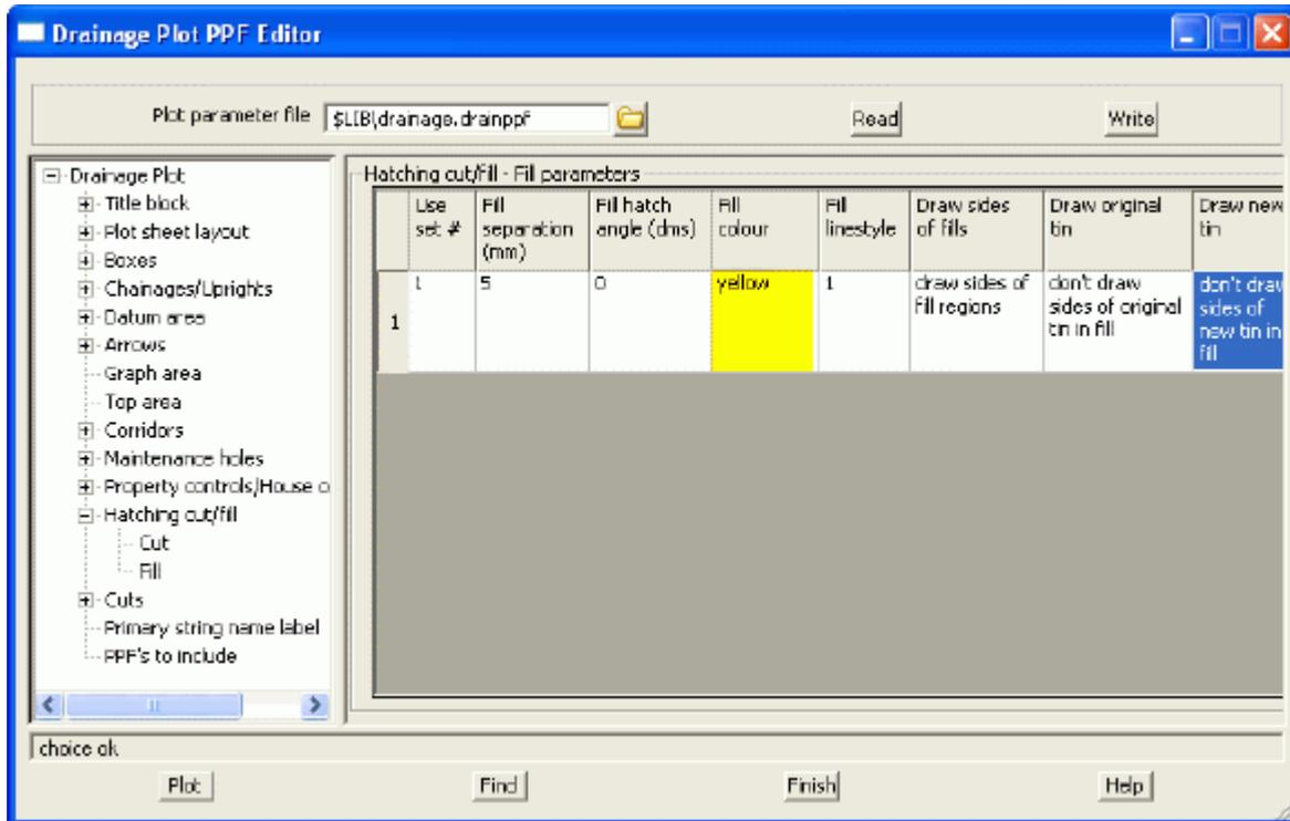
Use set # is entered as 1. **Fill separation, hatch angle, colour and linestyle** selected as desired. **Draw sides of tin, Draw original tin** and **Draw new tin** are not required unless you want these extra line in the drawing.
